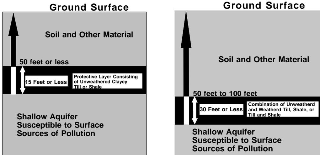
**SHALLOW WELL** - A well which is completed in a shallow aquifer.
